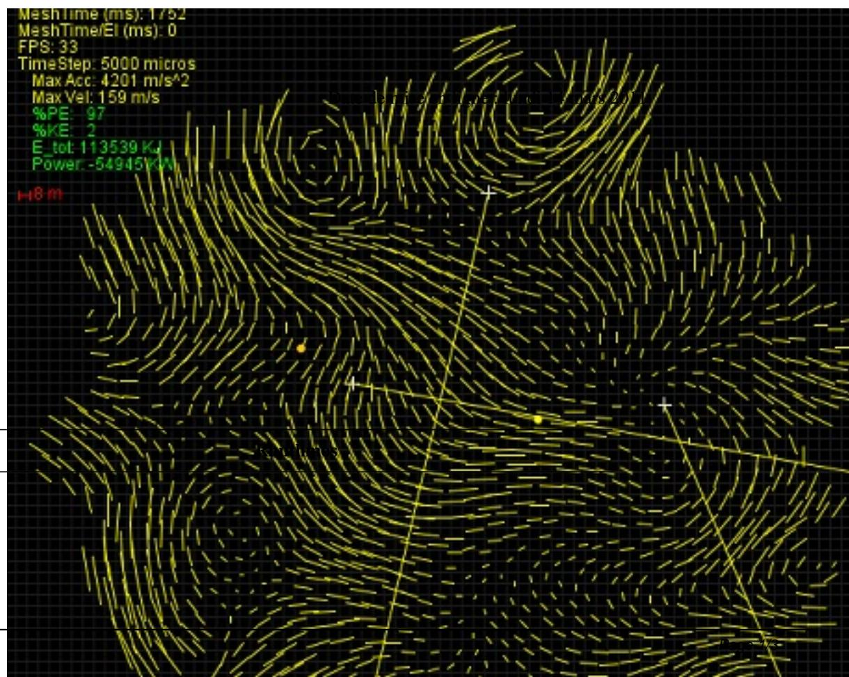
Usage : Choose your demo. Use your mouse or type commands into the textbox prompt at the top of the applet. This includes the ability to multi-select elements by right-dragging. You can then selectively apply mass and stiffness using « m [mass] » and « k [stiffness] ». To fix selected elements type « fix »
